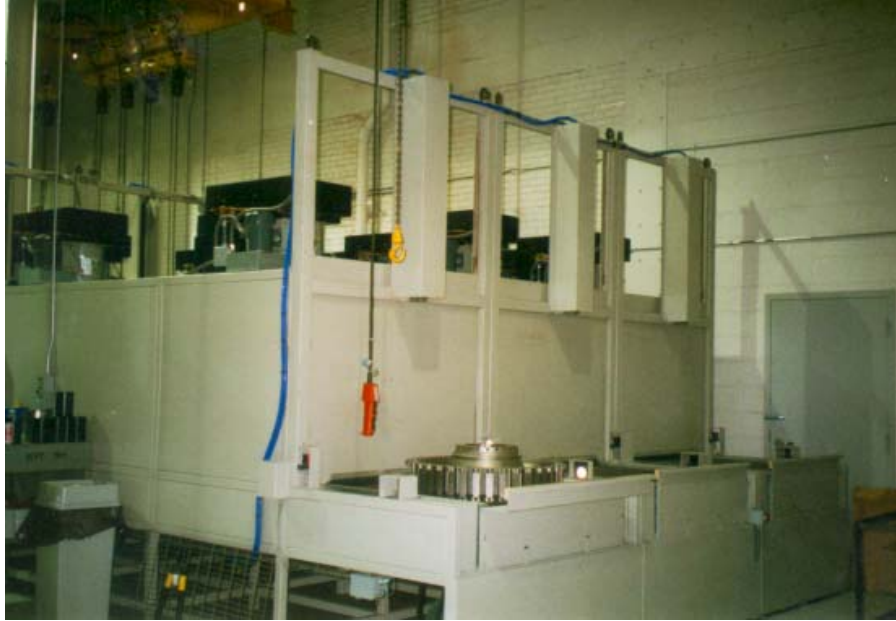
Figure 3. Oven dry facilities made available for the study. The far oven of this three oven furnace was utilized for all oven dry steps. Each of the three ovens is independently controlled.
