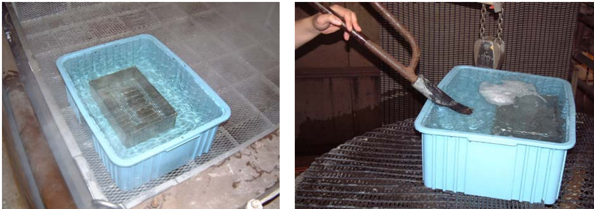
Figure 2. Hot water rinse tank used for wetting the samples and for the flash dry method. The left image shows the samples in the basket which was placed inside of a plastic container and submerged in the hot water rinse tank. The right image shows the samples being cooled back to ambient temperature using a cold water rinse. This same tank was used for the flash dry method and was operated at 185°F throughout the study.
